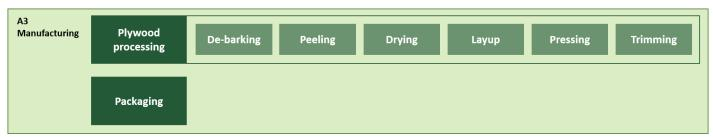
Figure 2. Softwood plywood manufacturing process
