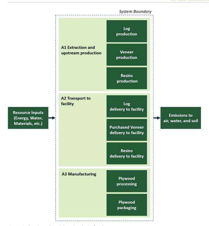
Figure 1. Cradle-to-Gate softwood plywood production flow diagram
