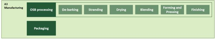
Figure 2. OSB manufacturing process
