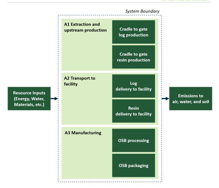
Figure 1. Cradle-to-Gate OSB production flow diagram
