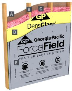
Illustration above is typical 1 hour fire rated assembly with fire exposure from both sides\*
