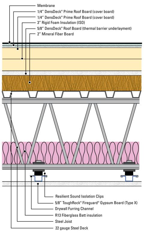
Tests per ASTM E 90 and ASTM E 413, were conducted in 2011 at Riverbank Acoustical Laboratories. Results are based on characteristics, properties and performance of materials and systems obtained under controlled test conditions. Actual results may vary.
