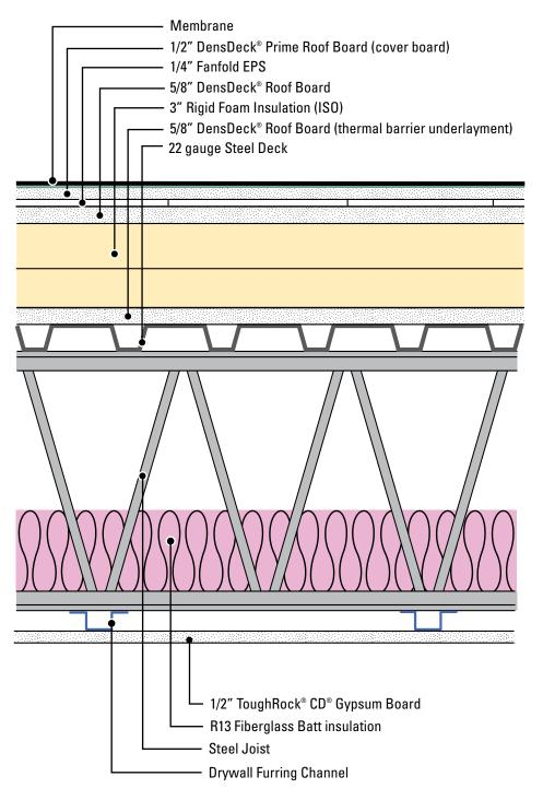
Tests per ASTM E 90 and ASTM E 413, were conducted in 2011 at Riverbank Acoustical Laboratories. Results are based on characteristics, properties and performance of materials and systems obtained under controlled test conditions. Actual results may vary.
