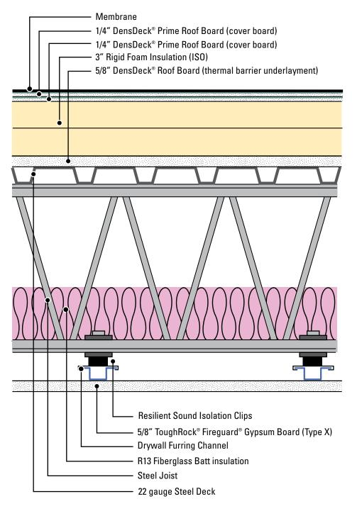
Tests per ASTM E 90 and ASTM E 413, were conducted in 2011 at Riverbank Acoustical Laboratories. Results are based on characteristics, properties and performance of materials and systems obtained under controlled test conditions. Actual results may vary.
