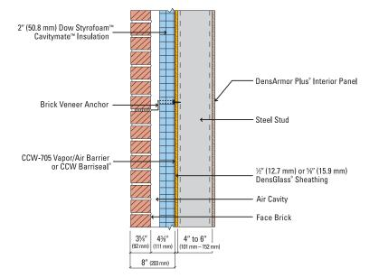
Note: CCW Primer is required for the CCW-705 Vapor/Air Barrier.
