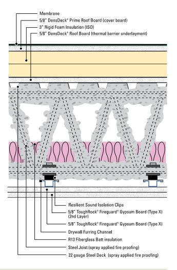
As shown in **Diagram #1**, the tested assembly consisted of a structural steel joist framing system and 22 gauge metal deck with a suspended ½" drywall ceiling. A ½" DensDeck® thermal barrier was installed over the steel deck and 3" of isocyanurate foam insulation with a ½" DensDeck® Prime cover board was placed over the thermal barrier. A 45-mil TPO membrane was then adhered to the DensDeck Prime.
