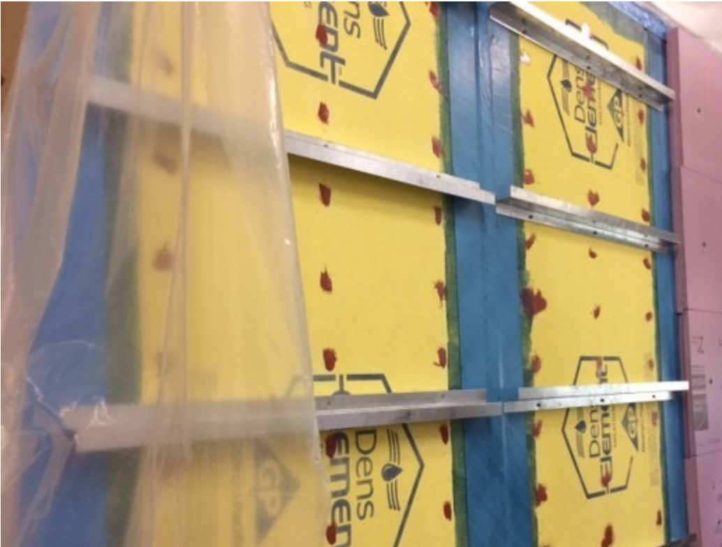
Picture 1: The DensElement™ Barrier System with Z Girts installed with flanges up and down. The Z Girts are installed both tight and spaced from the WRB. Far right test wall shows XPS attached.
