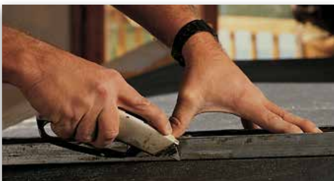
Cutting is a snap! Simply score and snap two sides with a single blade. And the cut edge will always be clean.
